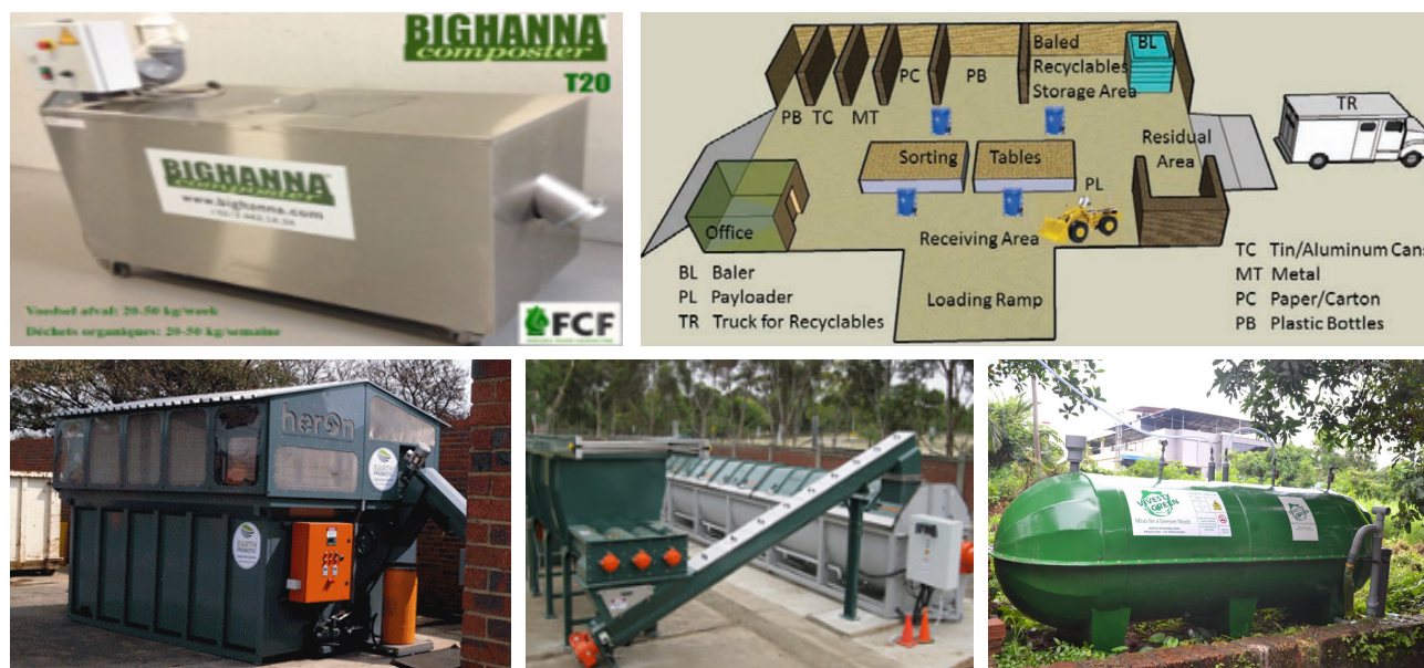
Figure 10: Examples of containerized composting (left-up, left-down, and middle-down), small-scale material recovery and transfer station (right-up), 2 and small-scale bio-digester (right-down) 3
